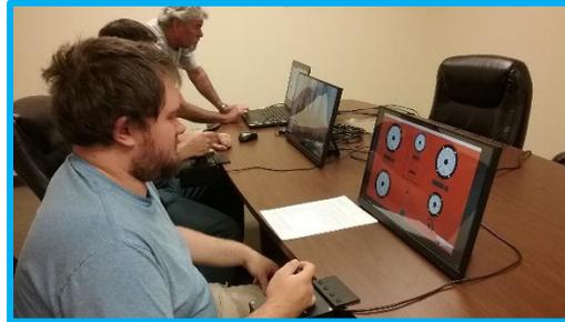
Included in this simulator package is an instructor laptop computer, 2 each 22-inch touch screen HMI (Human Machine Interface) monitors and 2 joy sticks.
