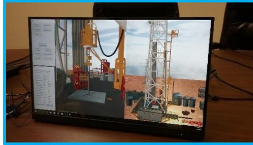
The Supervisor uses an HMI to interact with the choke gauges and controls that are used on a remote choke. The Supervisor also has a joy stick used to open and close the choke during well control scenarios. This simulator is packaged in a single small light weight pelican case that is durable enough for shipping and airport handling. Two mounting brackets are included for table top mounting of the joy sticks.
